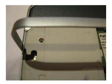
6. Install the Mini SD connector in the mini SD slot first. To do this with the cable connected to it you will have to pull the door all the way until it stops and bend it down then insert the Mini SD connector with the cable hanging out. Insert it the same way you would a mini SD card. It should click in the same way as the card usually does. **Push in to insert until the click push in again to remove it**. The gold contacts should face away from the screen. **Do not pull by black cable.**
