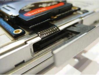
Also notice how the cable folds into the Mini SD slot to allow the extended part of this slot cover to go all the way in without hitting the cable. When the door is closed this fold will allow it to close tightly.
