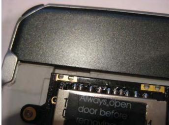
15. If it is miss-aligned you will have to remove the screw right away and lift up the screw side slowly until the tape becomes un-stuck. If it remains on the tablet this is ok just put the screw in again and try the alignment again.
