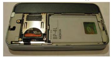
This is the finished installation of the adapter with the metal cover removed.
