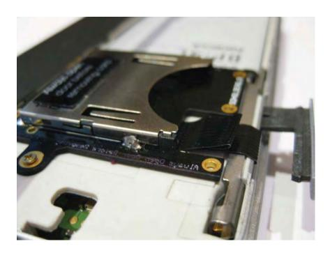
18. From the side the folds look like this (see photo above). Note how the fold around the N810 body from inside the Mini SD slot is close to the body. The other 2 folds are folded on top of each other. The do not have to be too tightly folded; just enough to be able to remove the SD card across the top of them. **Do not tape them down in any way**.
